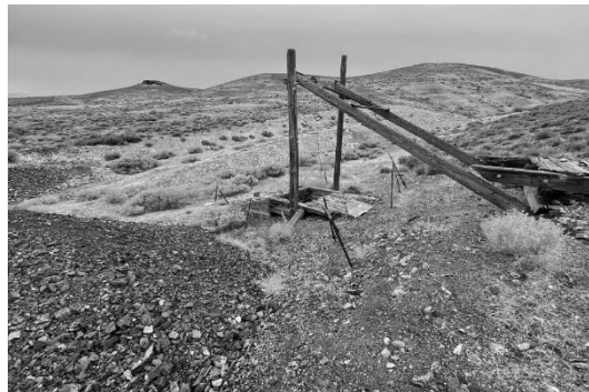
Figure 3. Historic Silver Coin headframe near utm N4531058 E472347. At this location, dump material is silicified, quartz veined, oxidized (limonite > hematite) and variable amounts of carbon. Exposed in the roadcut behind the headframe is weakly oxidized and bleached igneous material of the Iron Point intrusion.
